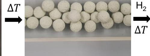
Calcined 3D-printed parts
